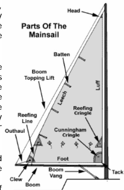
tighten the sail's luff (front edge of the sail) and move the draft forward and back to its correct position approximately 45% of the way back from the luff (front edge of the sail). To set the Cunningham, loosen the main sail halyard and pull the Cunningham cringle over the reefing hook.
