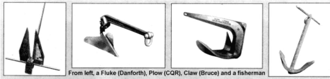
**Danforth anchors:** The lightweight anchor, such as the Danforth or Fortress, is a burying anchor with wide sharp flukes and a stock. It holds very well under high loads in mud and sand but may be difficult to set in clay, grass, weeds, rock or shell bottoms. You may want to consider a lightweight as a secondary working anchor or a lunch hook. It requires more scope than other anchors and can be stored flat on deck, or from a rail.
