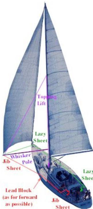
**Attachment to the Mast:** Mast attachment is critical to insure that the whisker pole can move in the necessary direction without binding under the compression loads. Mast fittings are available in two basic styles: fixed eye or sliding car.
