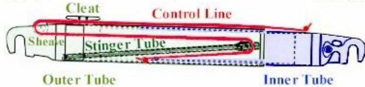
By un-cleating this line, you simply pull the line and the pole telescopes. To set the length you then cleat off the line when you've reached the desired length.
