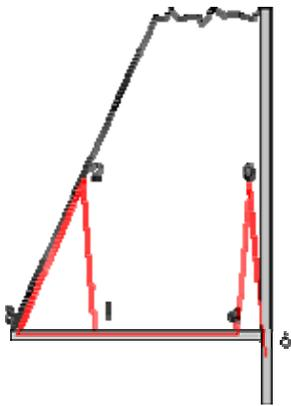
**These reefing lines should be tied around the bottom of the sail and ABOVE the boom. Tying them around the boom may cause the sail to rip in high winds.**
